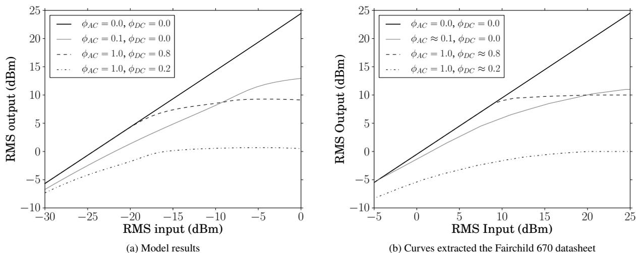
Figure 12: The static gain characteristics of the Fairchild 670 model (a), at various threshold levels, and data taken from the datasheet curves [15] (b). Notice that the range of the x-axis is different for the two plots; the gain at no limiting for the model is different than that reported by the datasheet.
