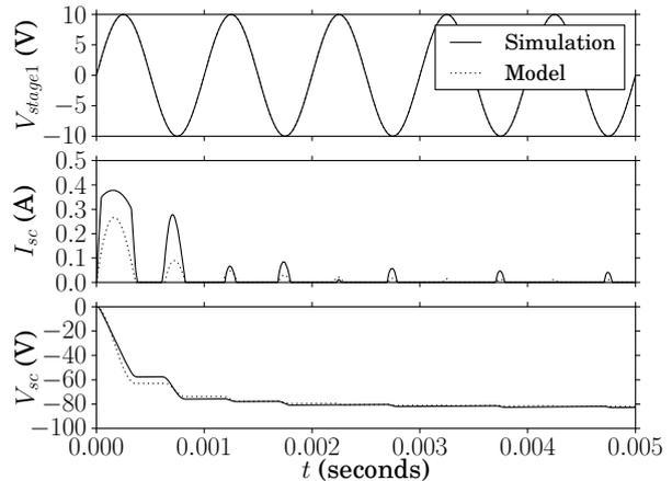
Figure 10: Simulation results for the second and third stages of the sidechain amplifier, compared with the model.
