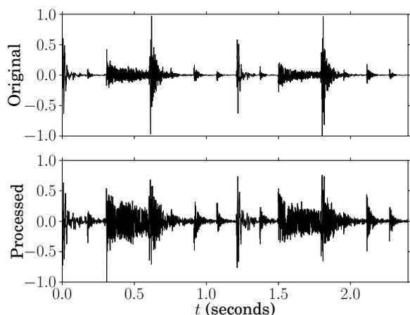
Figure 11: The top plot shows an acoustic drum loop and the bottom plot shows the loop processed by the model, with  $\phi_{AC} = 0.5$ ,  $\phi_{DC} = 0.1$ , and time constant 1, processed at 44.1 kHz with 8 $\times$  oversampling. Both plots have been normalised to the same peak value for easier visual comparison. Notice that the overall level of the processed audio is higher.
