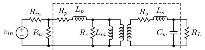
Figure 3: A transformer model (inside the dotted box) driven by a resistive voltage source with an input termination resistor and a resistive load.
