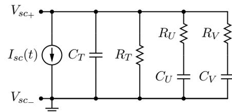
Figure 8: The sidechain time constant circuit. The component values are different for each position of a six-way switch.
