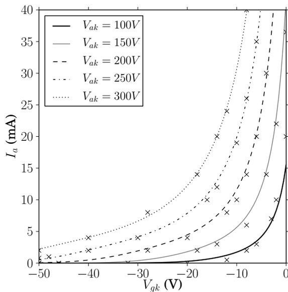
Figure 2: The modelled 6386 triode transfer characteristics. The points used to fit the curves were taken from the datasheet [6] and are shown with x’s.
