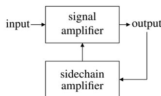
Figure 1: An overview of the Fairchild 670 circuit. The sidechain amplifier estimates the output level which is fed back to control the gain of the signal amplifier. This non-linear amplification limits the voltage of the peaks in the output.
