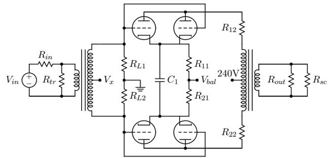
Figure 5: A simplified circuit diagram for the Fairchild 670 signal amplifier. The triodes are 6386s.
