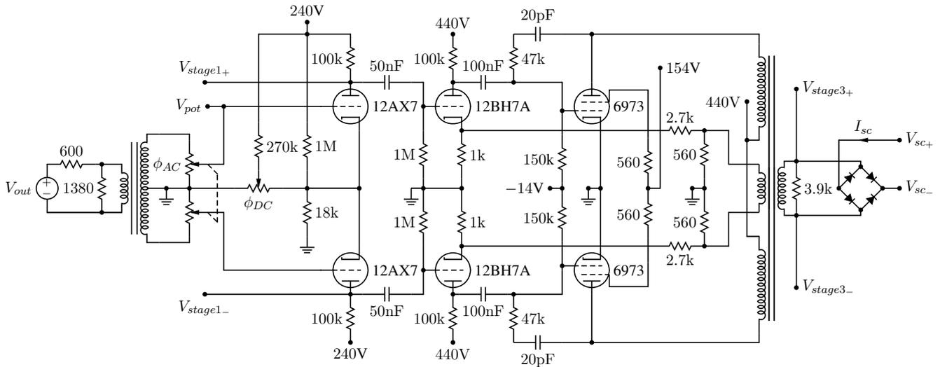
Figure 7: A simplified circuit diagram for the Fairchild 670 sidechain.
