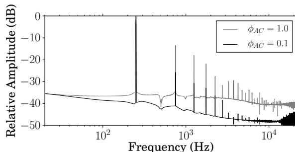
Figure 13: Spectra of the model output driven by a  $-3.8$  dBm, 250 Hz pure tone input, for two different AC threshold values, normalised for the fundamental to peak at 0 dB, processed at 44.1 kHz with 8 $\times$  oversampling. A higher AC threshold results in more gain reduction and higher distortion.
