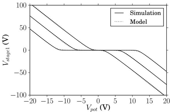
Figure 9: Simulation results for the first stage of the sidechain amplifier, compared with the model, for  $\phi_{DC} \in \{0.1, 0.5, 0.9\}$ .
