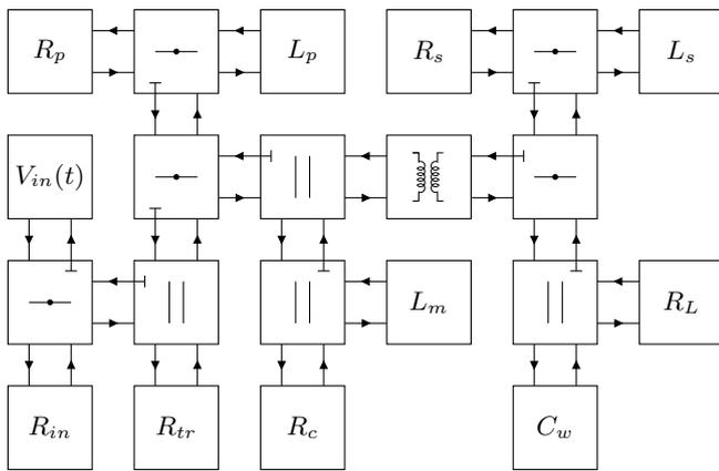
Figure 4: A wave digital filter transformer model driven by a resistive voltage source with an input termination resistor and a resistive load. In this figure, the transformer symbol represents an ideal transformer, with its primary coil on the left and its secondary on the right.
